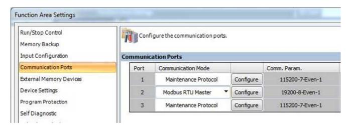
Set the communication Mode of the connected port to Modbus RTU Master, and push on the Configure button.
